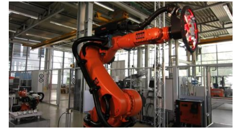
Worker assistant with high-payload industrial robots Manually guided robot/ safety/ ergonomics
