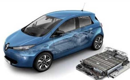
Zoé 400 V, 41 kWh, 12 modules, 192 cellules, 290 kg
