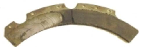
Fig. 6. Exemple de garniture endommagée - Example of damaged lining
